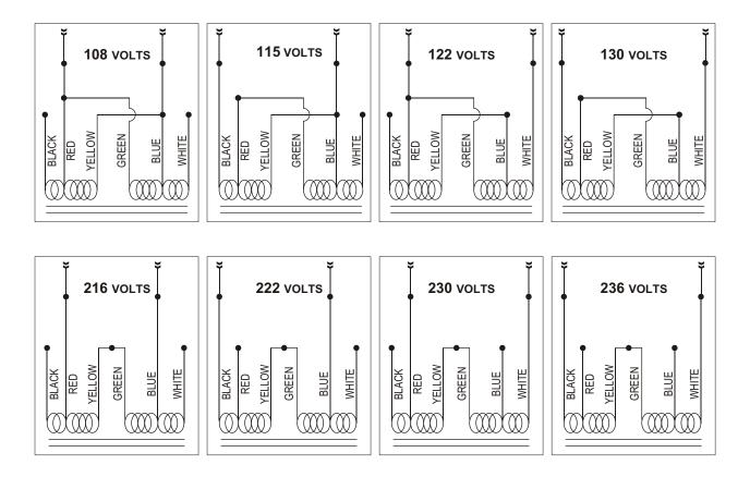
All the wire connections *including* the unused wires, should be well insulated with approved connectors, then double-insulated with electrical tape.
